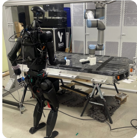
Fig. 1: A Unitree H1-2 humanoid working alongside the gantry-based RAPID disassembly cell [2] on a Hyundai Ioniq 5 battery pack. GOLEM augments automation infrastructure designed around human workers with humanoid autonomy.
